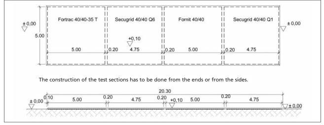
Figure 7. Plan and longitudinal section of the trial earthworks for the "Reinforced sub-base" field test.
