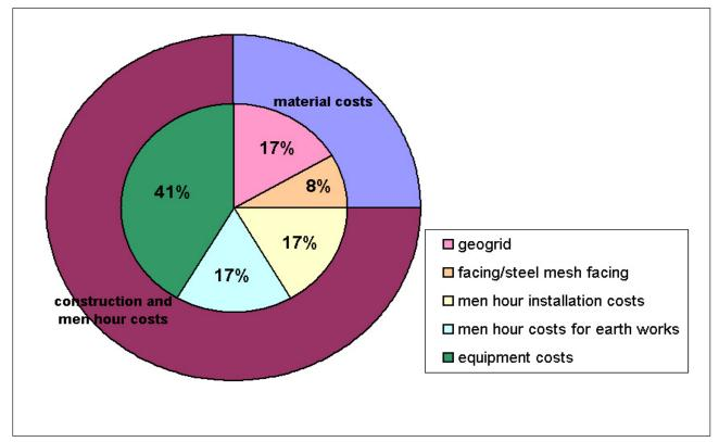
Fig. 2. Cost mix of a completed geosynthetic-reinforced earth structure
