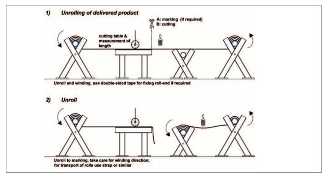
Fig. 12. principle of unrolling and winding station
