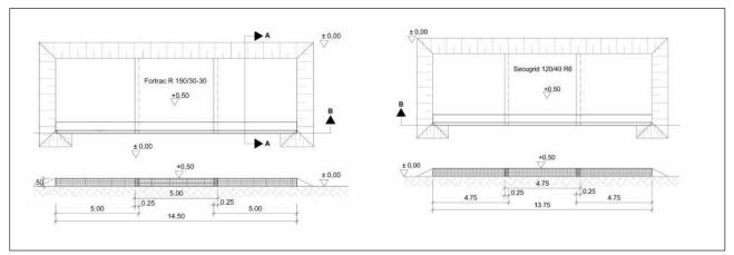
Fig. 4. Plan and longitudinal section of the trial earthworks for the "Steep reinforced soil slope" field test, left: Area 1 with flexible geogrid type 1, right: Area 2 with interlaced geogrid type 2.
