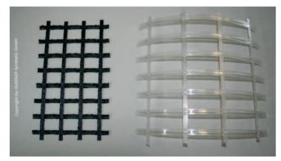
Fig. 5. Geogrids used in the "Steep reinforced soil slope" field test earthworks, left: Flexible high-modulus geogrid (type 1) right: interlaced, spot-bonded geogrid (type 2)
