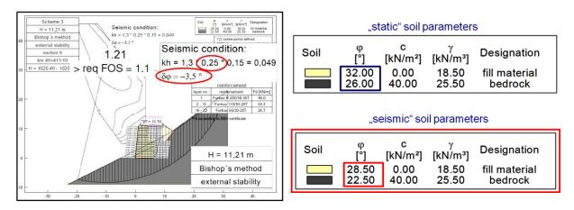
Figure 8. Seismic external stability analysis for the cross-section in Figure 6 (left); and assumed soil parameters right.
