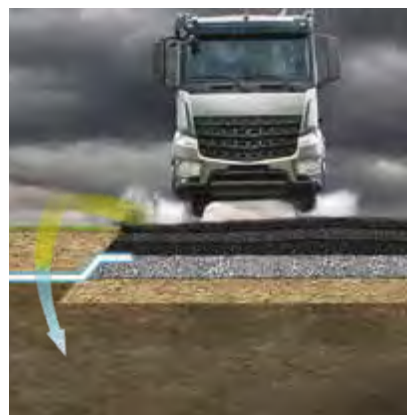
Decentralized precipitation treatment on roads
