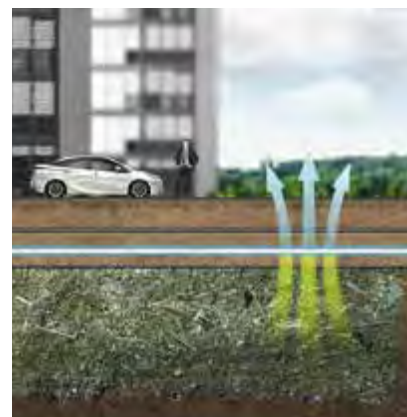
Soil air filter on contaminated sites
