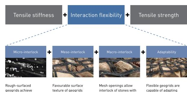
microscopic interlock with soil particles (friction).
