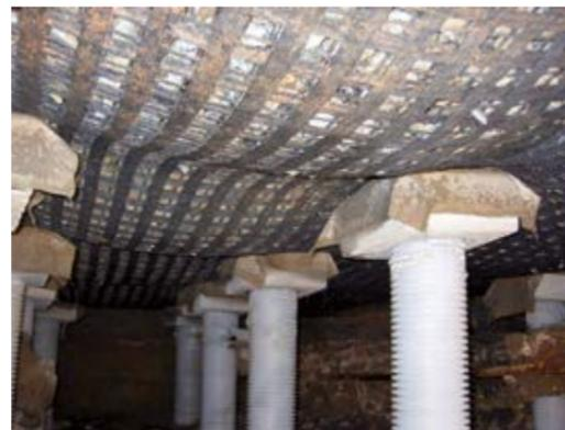
Membrane effect in piled embankment application
