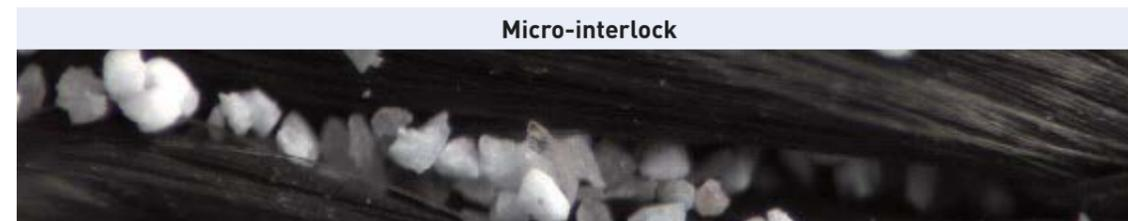
**Synonym for friction/adhesion:** microscopic interlock of soil particles with grid surface.
