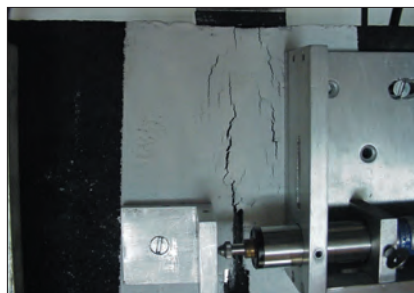
HaTelit® -reinforced specimen: bending failure after 490,000 cycles
