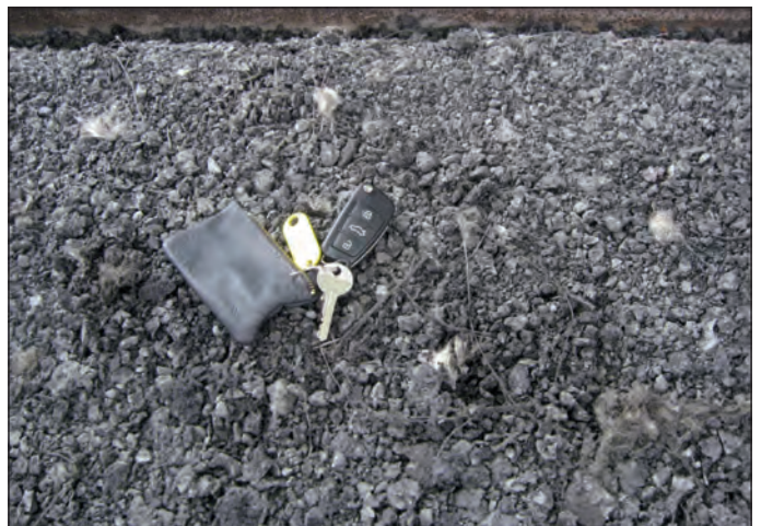
Small quantities of HaTelit® fibre residue in milled asphalt
