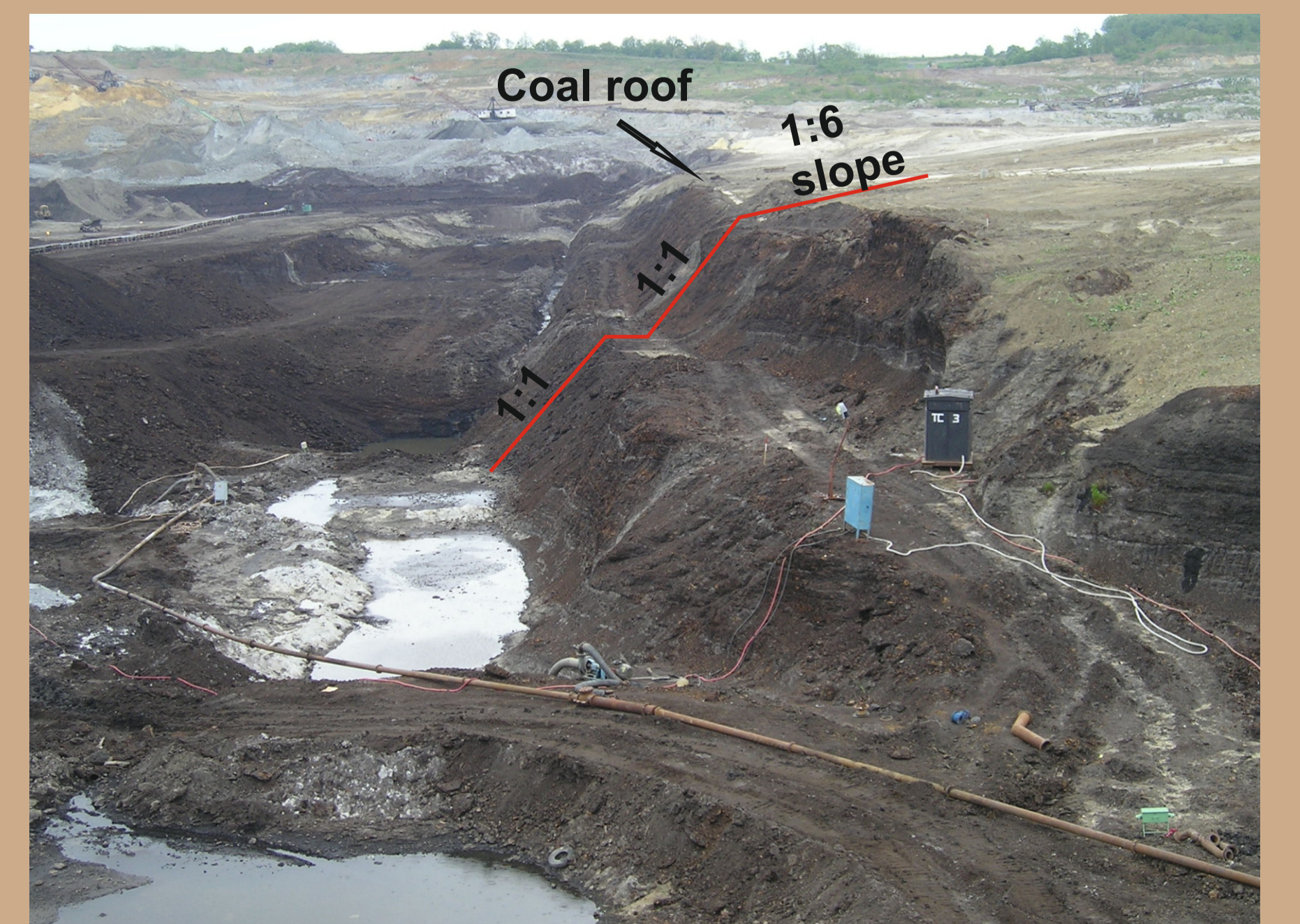
Coal excavation at the front after reopening of the coal mine in the field "B"
