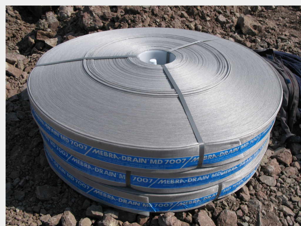
Horizontal installed geosynthetic drains in the spacing of 1.0 m on the base of working platform
