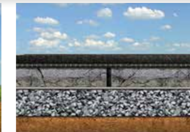
Rehabilitation of Concrete Pavements with Asphalt
