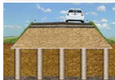
Geotextile Encased Columns (GEC)
