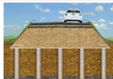
Geotextile Encased Columns
