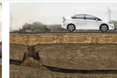
Bridging of Sinkholes
