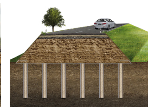
Embankments on Piles
