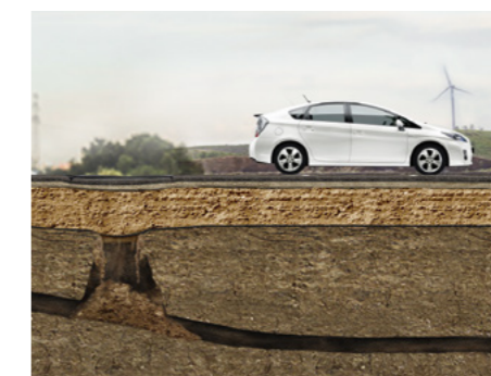
Bridging of Sinkholes
