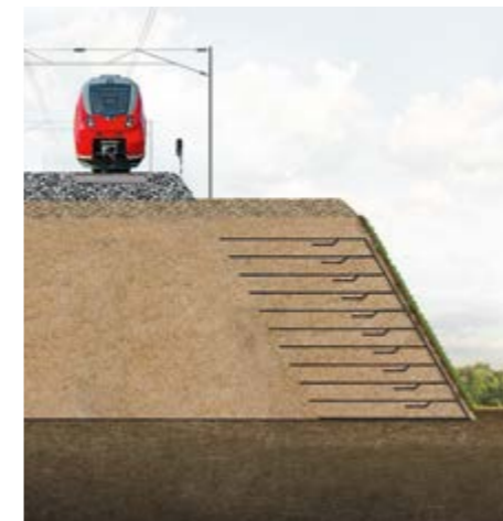
Retaining walls/steep slopes
