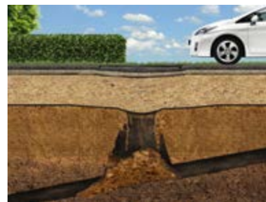
Bridging of Sinkholes
