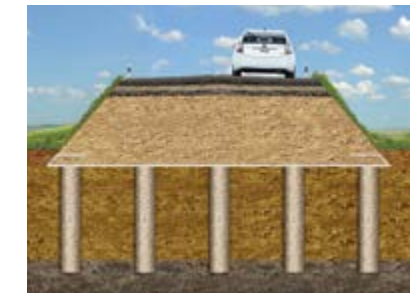
Geotextile Encased Columns (GEC)
