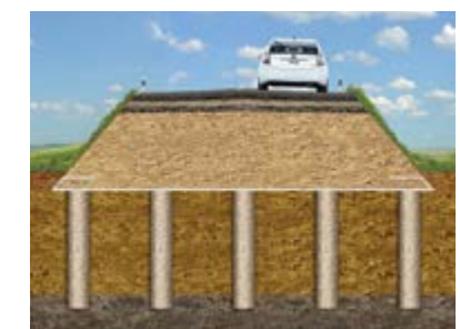
Geotextile Encased Columns
