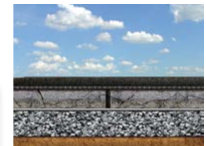
Rehabilitation of Concrete Pavements with Asphalt
