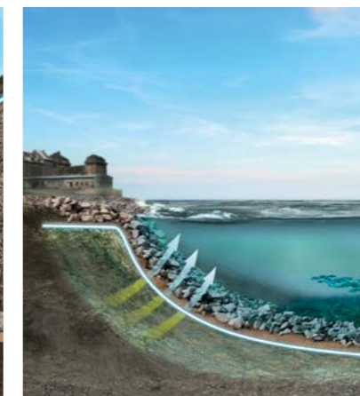
Isolation of contaminated sediments
