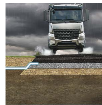
Decentralized runoff treatment on roads
