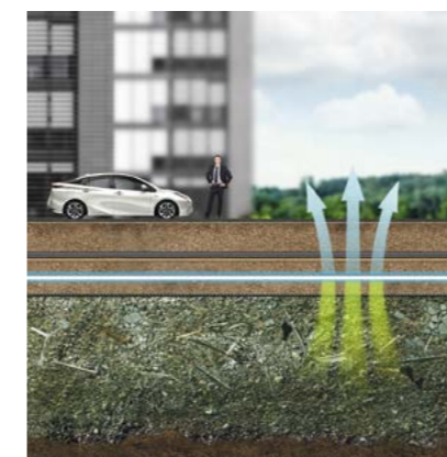
Soil air filter on contaminated sites
