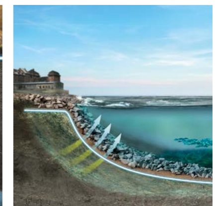
Isolation of contaminated sediments
