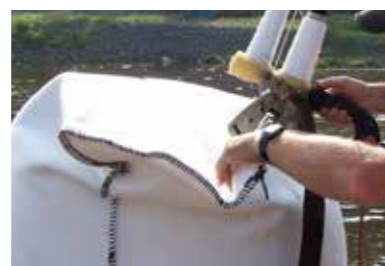
Closing of the bags by means of a hand held sewing machine
