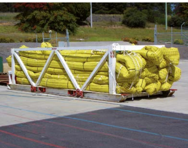
Longwall Recovery System crated for transport underground.
