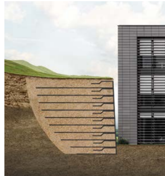
Lateral earth pressure containments
