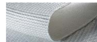
Stablenka® Reinforcement woven (PET) for soils with pH values from 2 to 9
